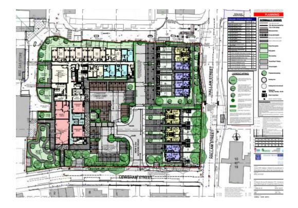
8.3 The proposed apartment block would be a maximum of seven storeys (equating to circa 23 metres height) and comprises red brick cladding facades and a contrasting colour to the ground floor, with accents of orange to the balcony features. Solar panels would be incorporated on the roof.
